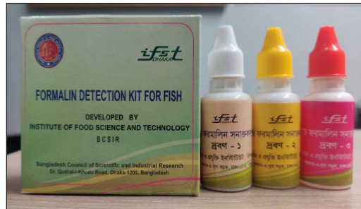
Figure 1. Bangladesh Council of Scientific and Industrial Research (BCSIR) kit for food formalin detection
